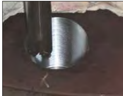
▲ New machined thread
