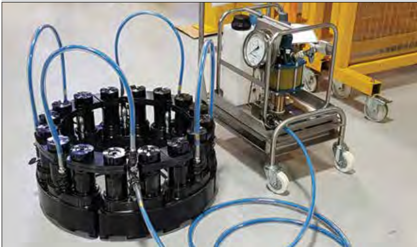
▲ Multi-Stud Tensioning Set-Up.
