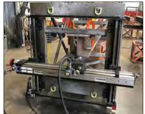
I-Beam end face milling with a GMRF1000. ▶
