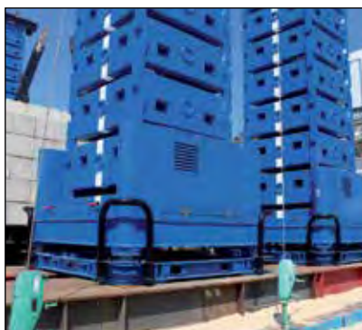
▼ Enerpac has been awarded a contract by Burkhalter to extend the height of Enerpac's 2200 ton (550 ton per tower) jack-up system from 66 to 118 feet for future projects.
