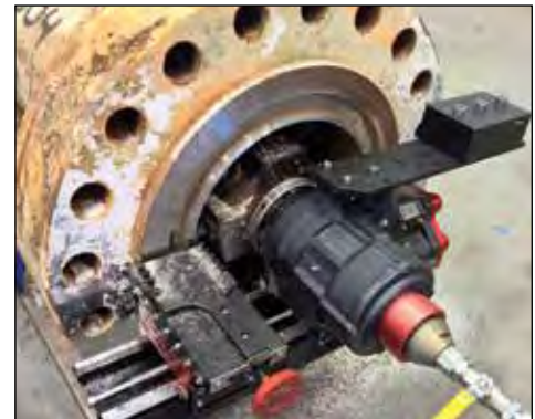
▼ MM860I machine to ensure flange joint integrity.
