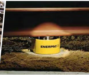
The TL248 Track Lift System can be deployed to lift rail bridge ends with included cylinders, or if needed, can operate hydraulic cylinders of other sizes.
