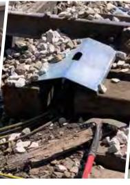
The TL248 Track Lift System includes four Ballast Shields to protect the lifting cylinders.
